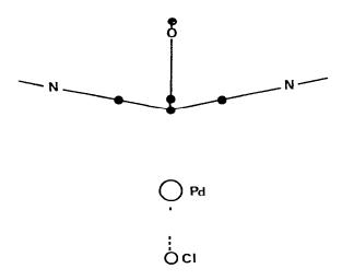
Fig 2 View do vn C(2)—C(4) showing the puckering of the cyclobutadiene ring of complex II
